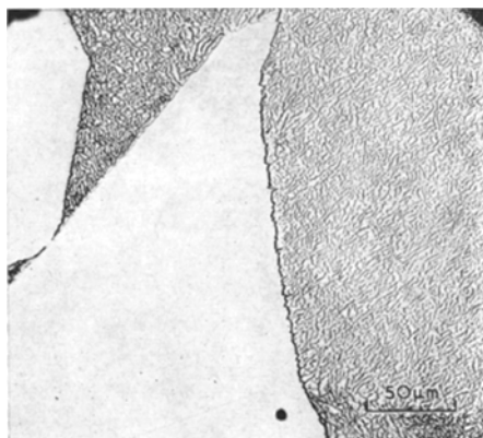
Figure 2 Microstructure of 69.3 mol % Al_2O_3 /30.7 mol % Y_3Al_5O_{12} composition solidified after heating to 1900° C. Temperature gradient = 190° C/cm, growth rate = 4 cm/h. Original magnification 500 ×.
