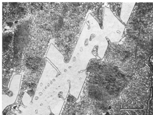
Figure 3 Microstructure of 85.7 mol % Al_2O_3 /14.3 mol % Y_3Al_5O_{12} composition solidified after heating to 1950° C. Temperature gradient = 190° C/cm, growth rate = 4 cm/h. Original magnification 500 ×.
